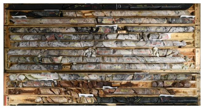
Figure 4: GTDD-22-0350 – example of coarse spodumene crystal laths within pegmatite mass (13.9m @ 1.53% Li<sub>2</sub>0)
